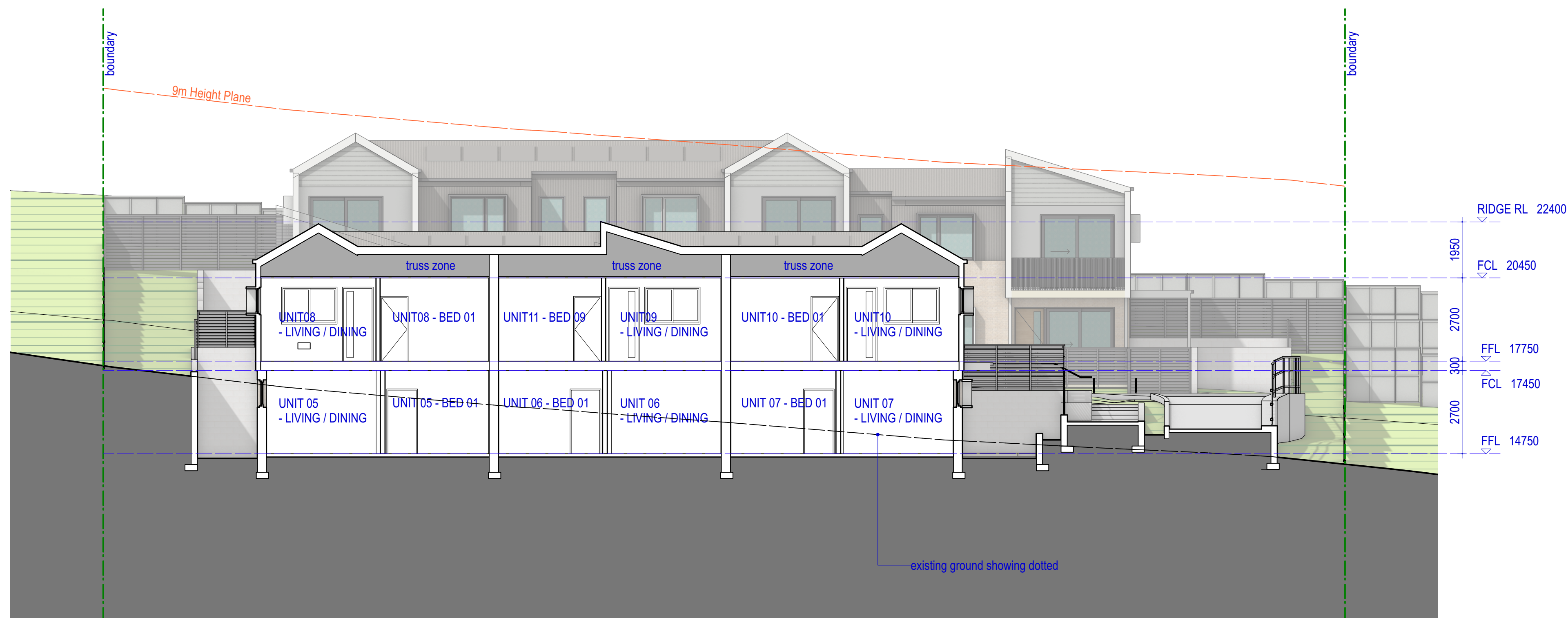
Architectural section drawing of a three-unit residential building. The drawing shows a cross-section of the building with three units labeled: UNIT 14 (Living/Dining), UNIT 15 (Living/Dining), and UNIT 16 (Living/Dining). Each unit has a bathroom (BATH) and a laundry room (LDY). The building features a truss roof structure. The ground level is indicated by a dashed line labeled "existing ground showing dotted". The drawing includes vertical dimensions on the right side: 1950, 2700, 300, 2700, and 17100. The drawing is bounded by a "boundary" line on the left and right. A "9m Height Plane" is indicated by a dashed line at the top left.
